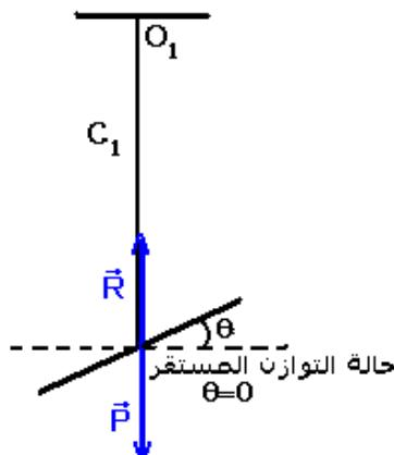
$$T'_0 = 2\pi \sqrt{\frac{z(L-z)J_{\Delta}}{L^2 \cdot C}} = \frac{T_0}{L} \sqrt{z(L-z)}$$
